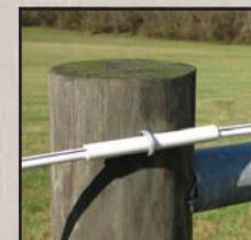
HOTCOTE® TUBE INSULATOR The strongest insulator available, being inside the staple. Use the extra wide 2" (50mm) barbed staples, which should be driven in so they allow the wire to move. Available in white, black and brown in 5" (133mm) lengths
